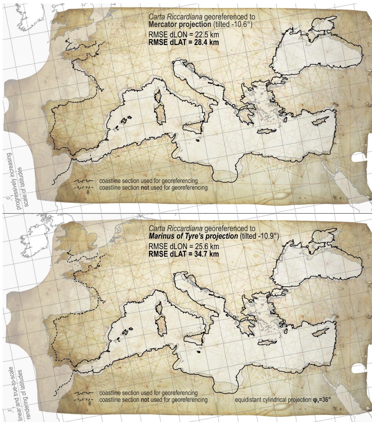
Figure 7: Rectified digitised images of the anonymous Carta Riccardiana portolan chart (c. 1300–1325) georeferenced to a modern map in the Mercator projection (the upper part) and to a map in Marinus of Tyre's projection (the lower part), with their proprietary axial RMSE accuracy levels. The greater of the two values, representing the chart's planimetric accuracy, is put in bold. Chart source: Biblioteca Riccardiana , Florence, call no.: Ricc. 3827. Basemap shapefile source: marineregions.org (Claus et al., 2017).
