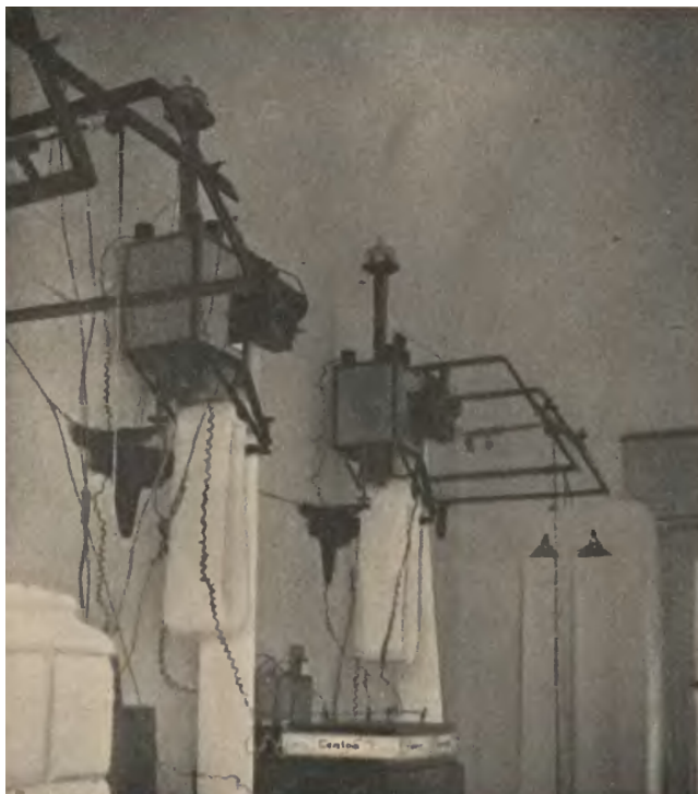
Figure 4. Inside of the atmospheric electricity measurement house with a view on two installed Benndorf electrometers hanged on the wall with brackets. The casing of each electrometer is earthed, and its plate electrodes are connected to a battery standing on the floor. The electrometers' needles are connected to wires coming from the outside, themselves connected to radioactive probes. Photograph from Szpecht (1939), page 214 (public domain).
