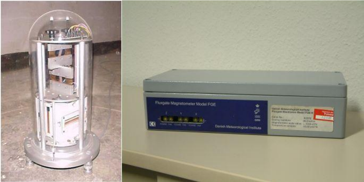
1 2 Fig. 20. Fluxgate magnetometer FGE sensor (left) and electronic unit (right). Source: 3 Helmholtz Centre Potsdam – GFZ.
