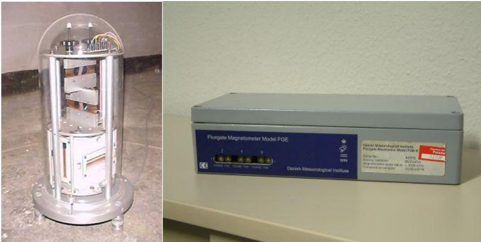
1 2 Fig. 20. Fluxgate magnetometer FGE sensor (left) and electronic unit (right). Source: 3 Helmholtz Centre Potsdam – GFZ. 4 5
