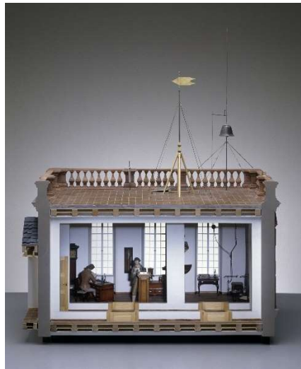
1055 Figure 4: Central station of the Societas Meteorologica Palatina in the Castle of Mannheim (historical situation showing the city wall, the castle and parts of the adjacent city). A model of the meteorological cabinet is available in TECHNOSEUM Mannheim (photo: Klaus Luginsland). The antenna of the atmospheric electrometer is seen on the roof to the right of the wind vane.
