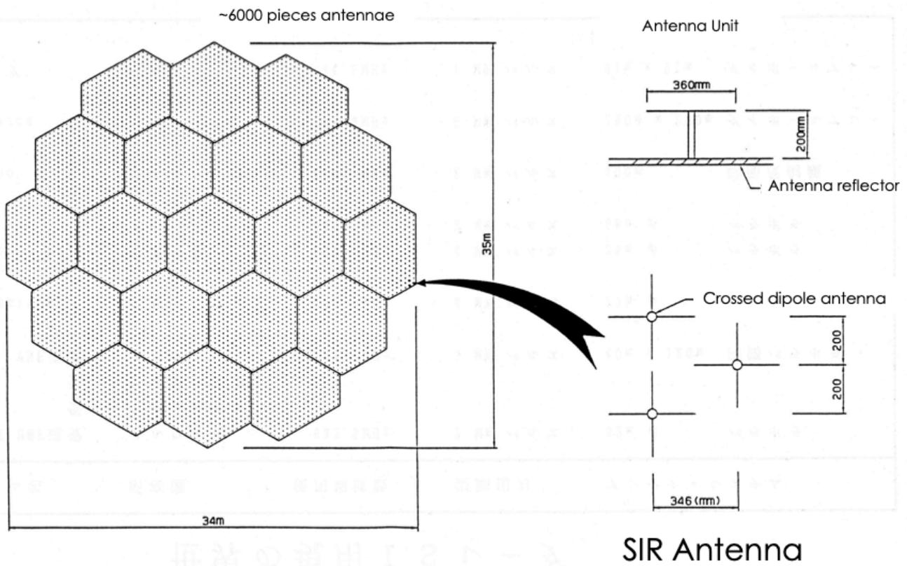
325 **Figure 2: The structure of the SIR phased array antennae. (Matuura et al., 1990)**
