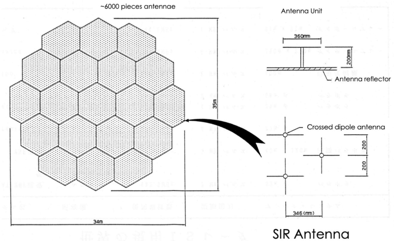
325 **Figure 2: The structure of the SIR phased array antennae. (Matuura et al., 1990)**
