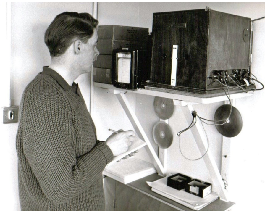
Figure 6. Readings being taken from the Brewer valve electrometer's chart recorder, by Monty Georgeson, a scientific assistant at Lerwick Observatory from 1966. Photograph from Lerwick Observatory archive.
