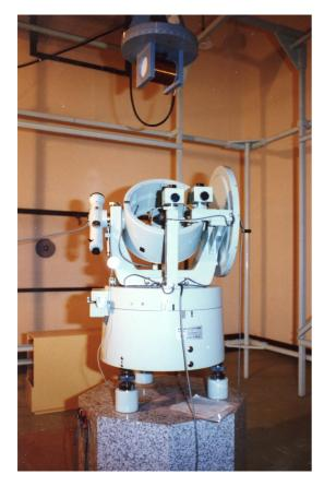
Figure 24: Newly developed theodolite DI72 beneath a proton processor magnetometer (photo supplied by Kakioka Magnetic Observatory).
