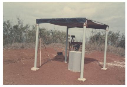
Figure 23: The pillar for the absolute measurement at Chichijima Magnetic Observatory (photo supplied by Kakioka Magnetic Observatory).
