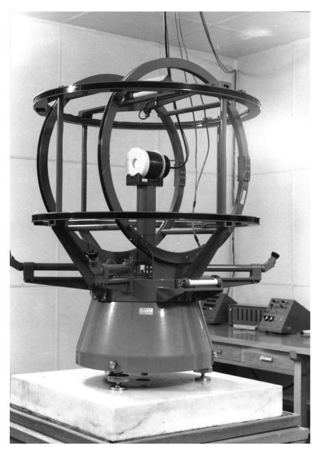
Figure 22: MO-P theodolite (photo supplied by Kakioka Magnetic Observatory).
