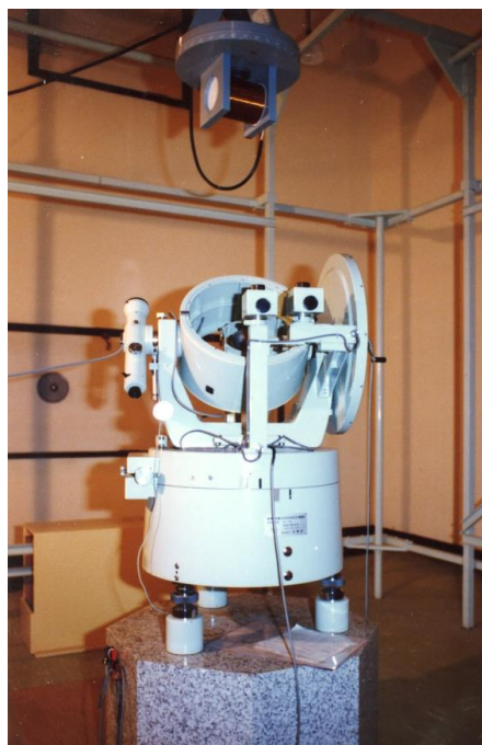
Figure 24: Newly developed theodolite DI72 beneath a proton processor magnetometer (photo supplied by Kakioka Magnetic Observatory).
