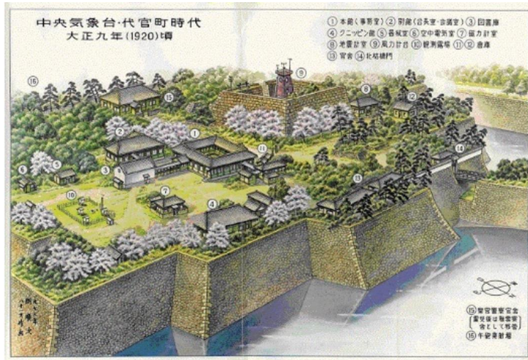
Figure 2: Central Meteorological Observatory at Kitanomaru of Edo castle. The building numbered as 7 is for the geomagnetic observation and that as 6 is for the atmospheric electric field observation (map supplied by Japan Meteorological Agency).
