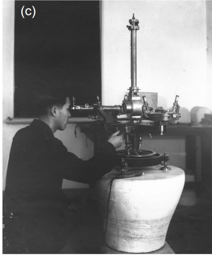
Figure 10: (a) Eshenhagen-Schmitt variometers, (b) an Indian survey pattern magnetometer, and (c) a Schmitt theodolite for the declination during an observation in 1952 (photo supplied by Kakioka Magnetic Observatory).
