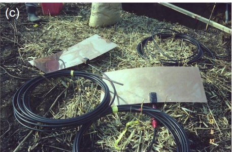
Figure 14: (a) a reflecting galvanometer and a voltmeter with a 10kΩ resistor, (b) cables, (c) a pair of the copper plate electrodes, and (d) a carbon rod electrode (photo supplied by Kakioka Magnetic Observatory).
