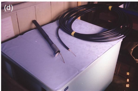
Figure 14: (a) a reflecting galvanometer and a voltmeter with a 10kΩ resistor, (b) cables, (c) a pair of the copper plate electrodes, and (d) a carbon rod electrode (photo supplied by Kakioka Magnetic Observatory).
