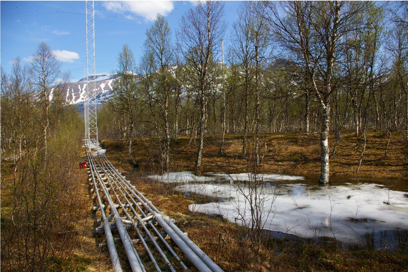
Figure 3: The fabricated coaxial cable and towers in one row of antennas of Array-2 in Spring of 2010. The vertical tubes which are part of the tower supporting the antenna are also coaxial cables acting as quarter wave transformers supplying the 130 RF current to the antenna. Array-3 has an identical design but is smaller in size. Originally Array-1 had similar antennas, larger in size, but these were modified after the storm in 1985. (Photo M. T. Rietveld)
