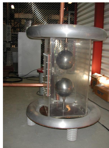
290 Figure 1: Left, an overview over part of the capacitor bank. Right, the "crowbar" spark gap. Photo courtesy of Ralf Larsen, Tromsø, formerly with EISCAT.
