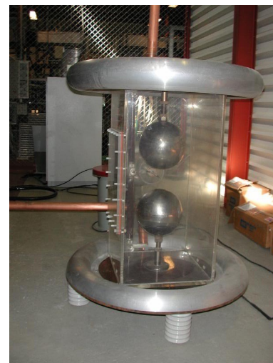
Figure 1: Left, an overview over part of the capacitor bank. Right, the "crowbar" spark gap. Photo courtesy of Ralf Larsen, Tromsø, formerly with EISCAT.
