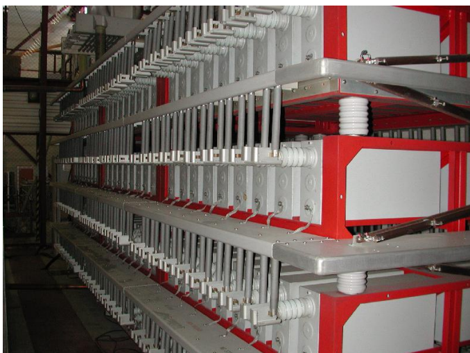
Figure 1: Left, an overview over part of the capacitor bank. Right, the "crowbar" spark gap. Photo courtesy of Ralf Larsen, Tromsø, formerly with EISCAT.
