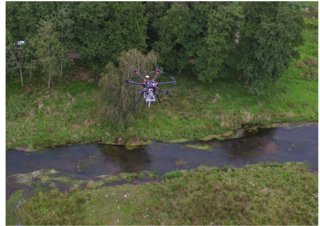
Figure 4. Flow measurements using a drone. Flight campaign by Sune Yde Nielsen, Henrik Karmisholt Grosen (Drone Systems.DK), Christian Josef Köppl and Filippo Bandini (DTU Environment).
