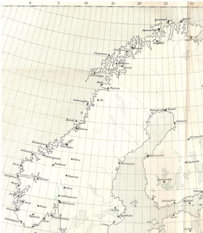
**Figure 3.** The first gravity network in Norway, established by pendulum observations by O. E. Schiøtz in 1892–1903. The locations around the Baltic Sea were measured by observers in other Nordic and Baltic countries.
