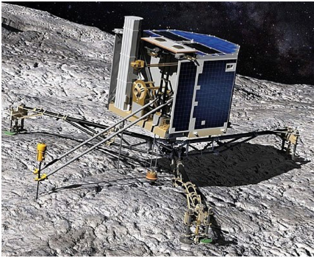
Figure 13. The Lander Philae of the Rosetta project. It was anchored to the comet by screws at the end of the three shock absorbing legs and contained ten scientific instruments (Source: DLR).
