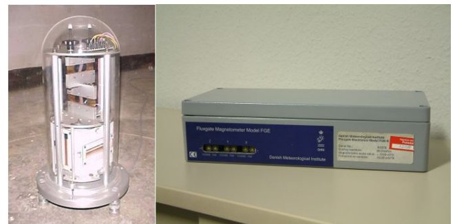
Figure 20. Fluxgate magnetometer FGE sensor (left) and electronic unit (right). Source: Helmholtz Centre Potsdam – GFZ.
